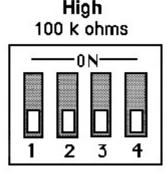
The "low" setting is for use with most direct-coupled solid-state preamplifiers such as those made by Jeff Rowland Design Group; the "medium" setting is for use with most solid-state, hybrid and some tube preamplifiers; the "high" setting is for use with most tube preamplifiers. We have provided these different settings so that you may find which one provides the best sonic results in your system. Your amp comes set from the factory at the "medium" (20 k ohms) adjustment.
