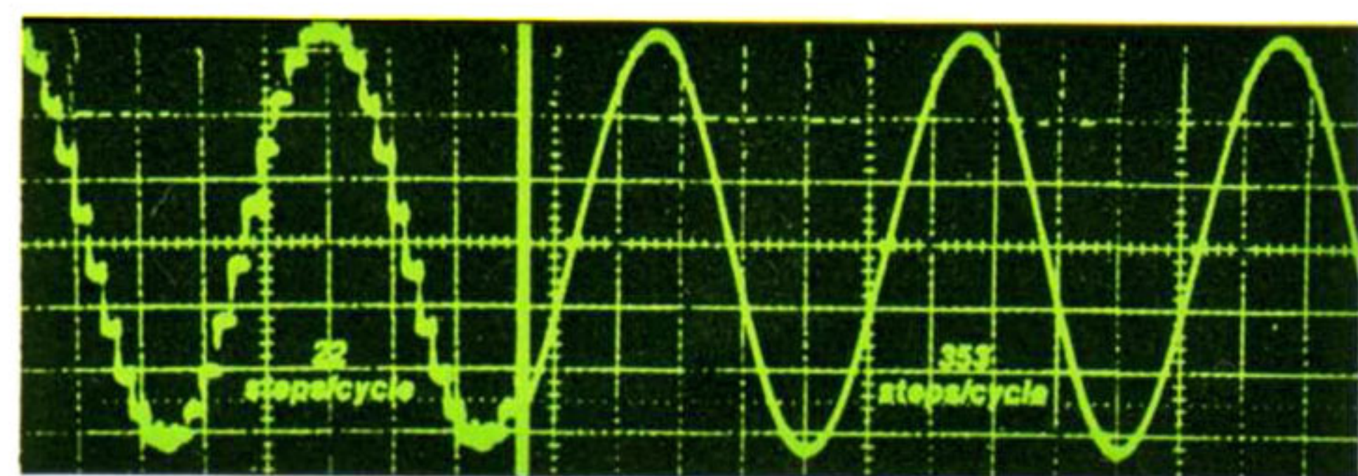
A comparison of 4-times (left) vs. Wadia 64-times resampling (right) reveals the smooth curve achieved . . . in this example, by 353 steps per 8 KHz cycle. As a result, the sharp peaks and gentle curves of every music waveform are faithfully recreated.
